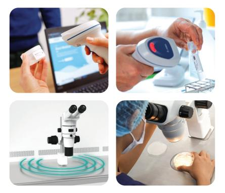
The MIRI® Evidence RFID traceability system uses hybrid human-readable RFID labels for the dishes to prevent mix-ups, allowing zero possibility for error. The MIRI® Evidence Pole reader automatically imparts 270° of coverage in the work area of the IVF workstation.
